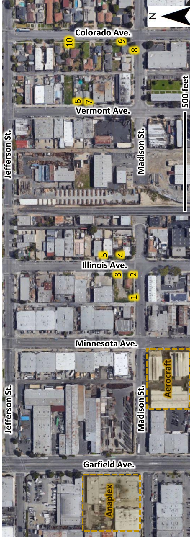
Figure 1: Locations of surface soil sampling near Aerocraft and Anaplex, Paramount, California.
