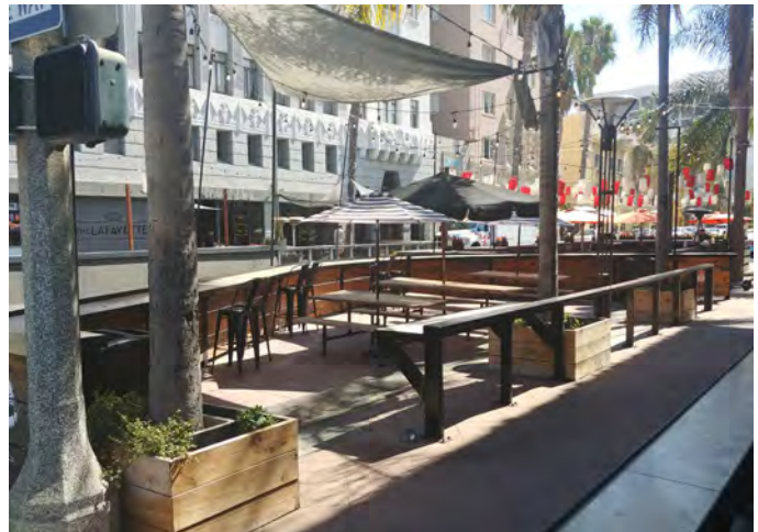
Parklet curb extension used to provide shaded outdoor dining areas in conditions where the building setback would not allow seating adjacent to the sidewalk
