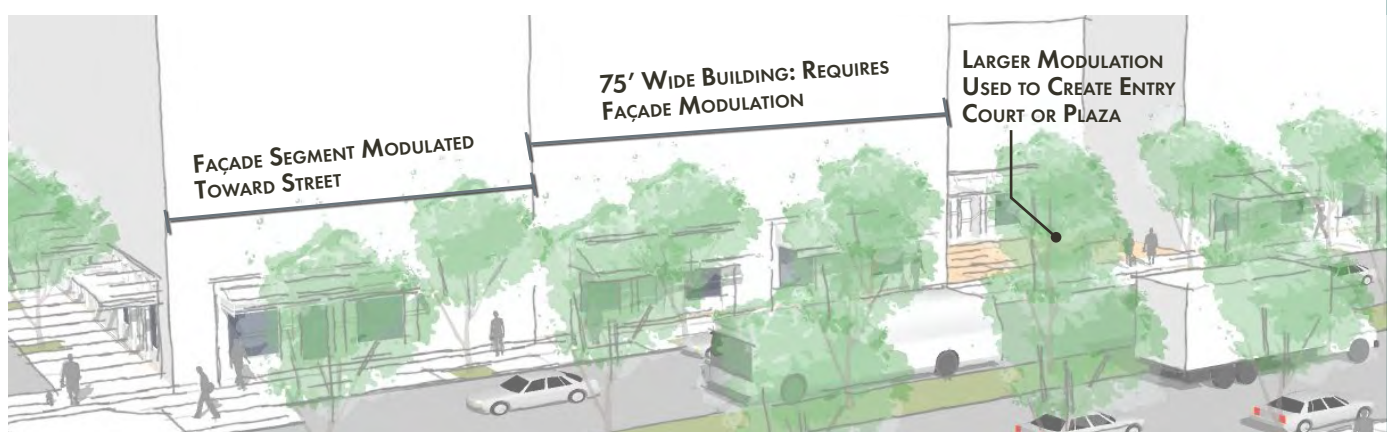
FIGURE 4.3 - ILLUSTRATION OF FAÇADE MODULATION
