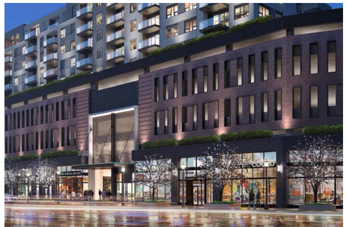
Structured parking visible above grade but included in mixed-use building with an architectural screen
