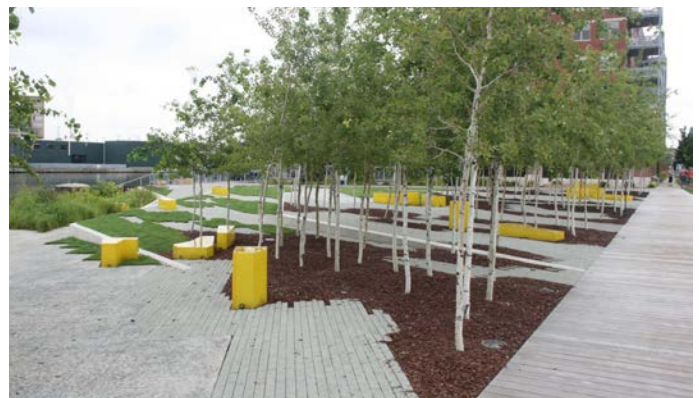
Erie Street Plaza, Milwaukee provides an example of a hardscape cap park that integrates landscape areas that provide phytoremediation.
