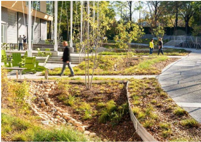
Bioswale and habitat planting within a plaza space that could be resident common space or publicly accessible plaza
